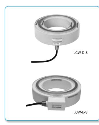
Hermetically-sealed structure with inert gas filled in ensures highly reliable, stable operation for a long period of time under harsh conditions. The flat washer-type structure requires only fabrication of screw nuts for installation to existing rolling mills.
