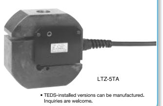
The LTZ-A series load cells adopt a Roberval's mechanism to ensure 1/3333 accuracy and easy handling and maintenance. Since they can be installed with less burden to existing facilities, they are used as compact, lightweight load cells with excellent cost performance for weighing or testing systems in various fields.
